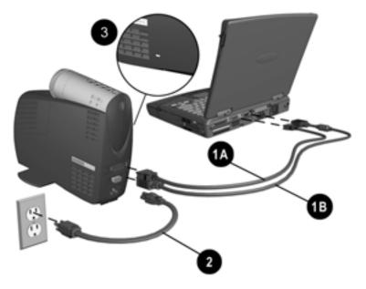
4. Press the blue Standby button on the top of the projector to turn on the projector first, then turn on the computer.
