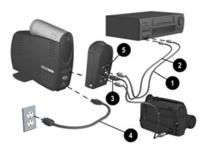
The Compaq Multimedia Adapter can remain attached to the projector, or it can be removed and stored in the carrying case.
