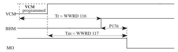
Tr = robot disengaging time in 1/10 s (WWRD 116)
