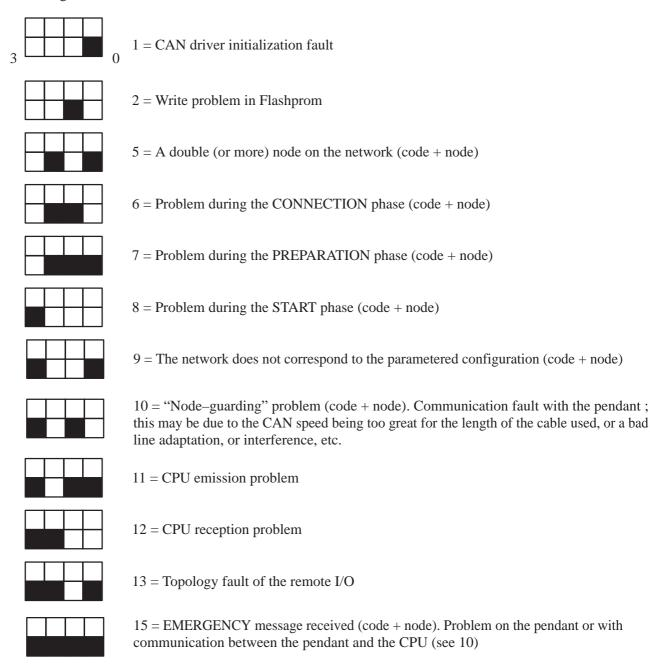
$\underline{\text{Note}}$ : In the event of a NODE GUARDING fault, fault 15 may appear alternately with fault 10.
