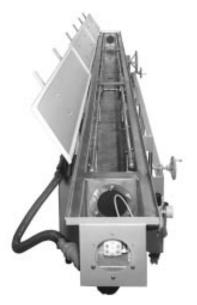
The extrusion passes from the water or spray compartment into an air-wipe compartment equipped with two, tubular air wiper rings connected to compressed air. Angled holes drilled in the wiper ring blasts air on the extrusion in the direction of the extruder to blow off surface water. A gasket seal at the exit of the air wipe compartment ensures the extrusion will be dry as it reaches the puller.
