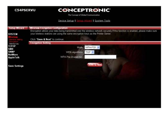
When "WPA-PSK", also named "WPA-shared key" requires users to select the advanced encryption methods, i.e. TKIP and enter a set of shared key.
