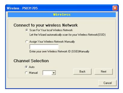
In the Ad-Hoc mode, you can let the print server automatically associate with other wireless station or manually assign the SSID of your wireless network. You can let the print server automatically select the channel that is the same with the peer or manually assign a channel.
