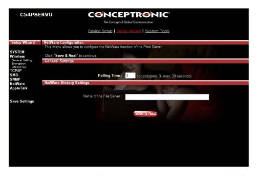
This print server supports NetWare Bindery Printing method. The print server periodically polls the NetWare server printer queues for printing jobs. You have to assign the NetWare server name, print server polling interval and the name of queue on the NetWare server for each printer port.
