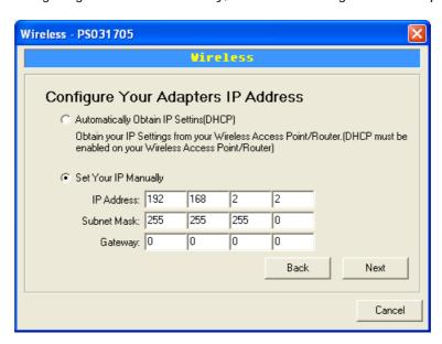
You can select to let the print server automatically obtain IP settings with DHCP client or manually assign the IP settings.
