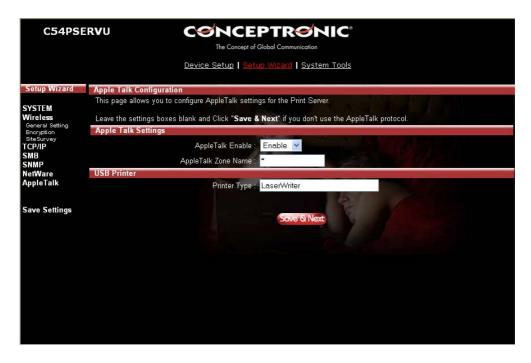
AppleTalk is a data communication protocol often used by Macintoshes. The print server can use these parameters to join the AppleTalk network and share the printer to other AppleTalk workstations. You have to select to enable or disable AppleTalk, and setup the "Zone Name" and "Printer Type" for each printer port of this print server.
