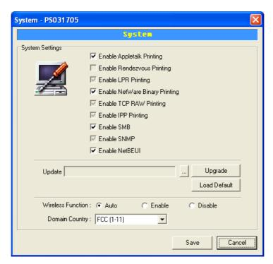
Double Click "System" icon and the System configuration window will pop-up. In the System configuration page, you can select to enable/disable each printing or management protocol, upgrade the new firmware for this print server, and enable/disable wireless function.
