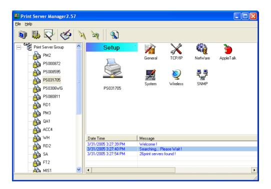
Every time when you run print server's configuration utility, click the "Search" icon on the tool bar. The configuration utility will delay for several seconds because the utility is using system's available network protocols to search for all print servers on the network. All available print servers will be listed under "Print Server Group" on the left side of the window.
