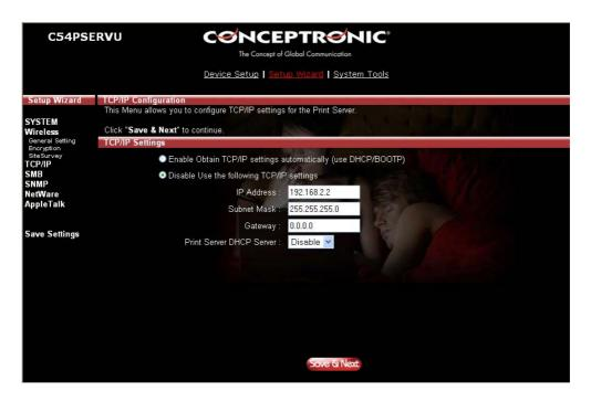
You can configure the print server to automatically get IP from DHCP server or manually specify static IP. The print server also has a built-in DHCP server. You can enable this DHCP server and let it manages IP for you.
