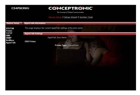
This page lists AppleTalk settings, including "AppleTalk Zone Name" and "Printer Type" of printers connected to all print ports.
