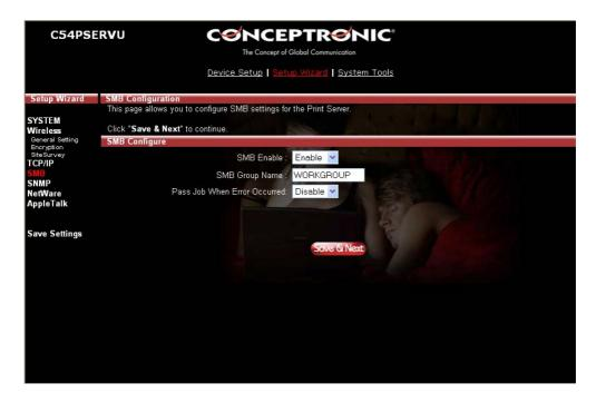
You can enable/disable the SMB protocol from here. If SMB is enabled, enter the "SMB Group Name" to specify the SMB group that this print server belongs to. All PC should join the same group before they can use this print server by SMB protocol.
