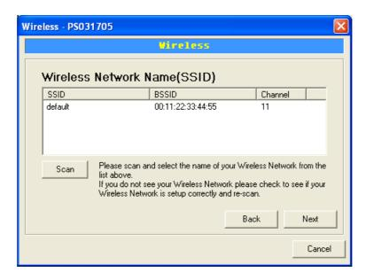
The list is the scanned active wireless stations. Select a wireless station in the list and click "Next". If you cannot find the wireless station that you want the print server to communicate with, click "Scan" to let the print server scan again.
