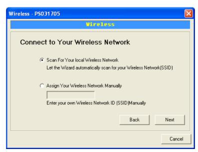
In the Infrastructure mode, you have to let the print server associate with an access point. You let the print server scan for an available access point automatically or manually assign the SSID of the access point you want to use.
