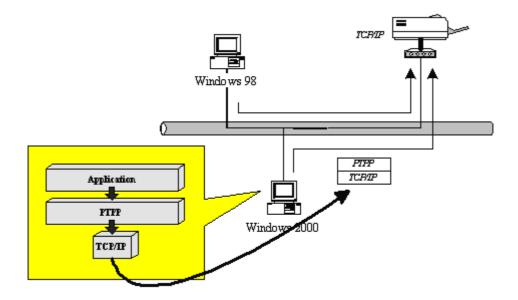
In the client installation procedure, after PTPP (Peer-to-Peer Printing Driver) is installed into Windows, the system will automatically (manual configuration is also allowed) search all the print servers on the network, and then add their printing ports into Windows' printing port (see below).
