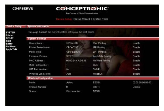
System Information includes "Device Name", "Print Server Name", "Model Type", "System Up Time", "Firmware Version", "MAC Address", "Wireless LAN Status" and the protocols enabled status, etc.
