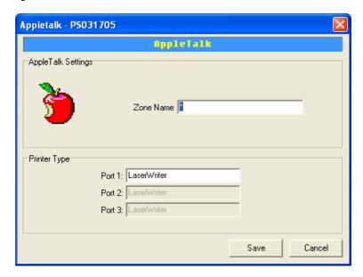
Double Click "AppleTalk" icon and the AppleTalk configuration window will pop-up. AppleTalk is a data communication protocol often used by Macintoshes. The print server can use these parameters to join the AppleTalk network and share the printer to other AppleTalk workstations. You have to setup the "Zone Name" and "Printer Type" for each printer port of this print server.
