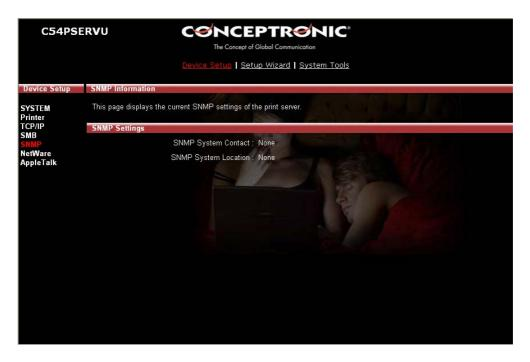
This page lists the SNMP settings of the print server. It includes the settings of "SNMP System Contact" and "SNMP System Location".
