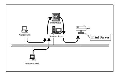
Compare with NetWare printing functionality, the advantages of embedding the NetWare network printing functionality in the print server include:
