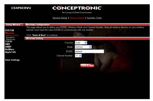
You can enable/disable the wireless function and set parameters that are used for the wireless stations to connect to this print server from here. The parameters include "Function", "Mode", "ESSID" and "Channel Number". You can manually set the parameters of wireless LAN in this page or use the "Site Survey" function to automatically search for an available access point and associate with it.
