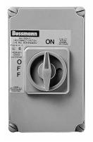
Catalog Symbol: BDNF30MS1 and BDNF60MS1 Ampere Rating: 30A, 60A Voltage Rating: 600V Enclosures: Valox® Handle: Nylon Agency Approvals: UL Standard, 508 – Industrial Control Equipment CSA Certified, C22.2 No. 14-M91 NEMA Type 3R, 4X, 12 VALOX is a registered trademark of GE Plastic Co.
