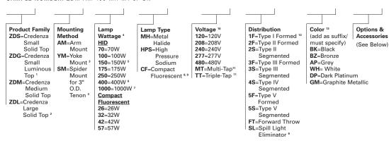
E.P.A. ZDS & ZDG: Arm Mount 1.19, Spider & Yoke Mount 1.13 / ZDM: Arm Mount 1.70, Spider & Yoke Mount 1.52 ZDL: Arm Mount 2.36, Spider & Yoke Mount 2.10
