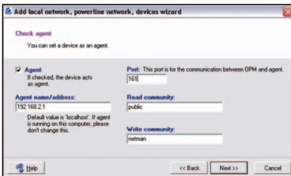
Fig. 3.49 Adding Powerline Device - Powerline Agent settings.
