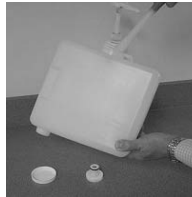
FIGURE 2. Remove Cap and Nozzle Adapter and Clean with Hot Water and Mild Dish Detergent using the Brush.
