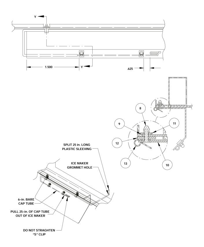
FIGURE 3. CAPILLARY TUBE LOCATION
