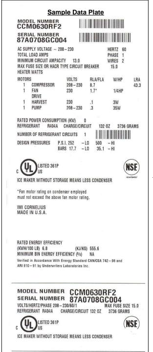
The serial number format and machine specifics are detailed on the data plate.
