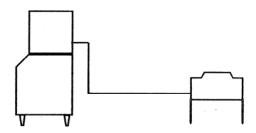
**DO NOT** Install the condenser lower than 6' (1.83 meters) below the quick connect fittings at rear of machine.
