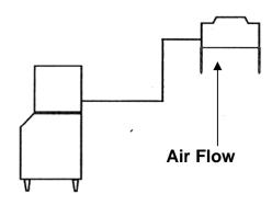
DO NOT Install any part of the refrigerant lines below the quick connect fittings at rear of machine.
