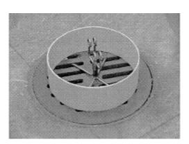
3. The adjustable clamps will accomodate 1/2– inch, 3/4–inch, and 1–inch I.D. either soft or ridgid (hard) PVC tubing. Squeezing the two tabs together that are located on the clamp–locking collar will loosen a tightened clamp.
