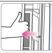
Please take out the plasma antibacterial catalysis filter, and then divide the filter into two pieces by pushing both hooks of the filter.
