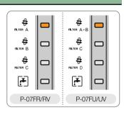
2 Each of A, B and C respectively represents Neo-sense filter, Membrane filter(RO), Fine Post-carbon filter.(P-07FR/RV) Each of A+B, C and D respectively Represents Plus-sediment filter+ Pre carbon Filter, Post carbon filter and UF Membrane filter.
