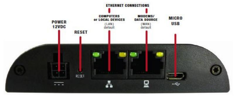
**Power 12VDC:** The power connector includes two pins for power and two pins for GPIO (General Purpose Input/Output) functionality. The included power adapter, however, only connects to the power pins. You will need a separate adapter for GPIO functionality.
