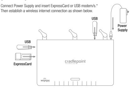
\*Only one Mobile Broadband Card is required to operate the MBR1000 as a wireless network in this setup. Mobile Broadband Card not included. See your Mobile Broadband Service Provider for details.
