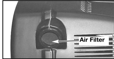
**IMPORTANT:** Do not operate the compressor with the air filter removed.
