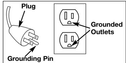
3. Inspect the plug and cord before each use. Do not use if there are signs of damage.
