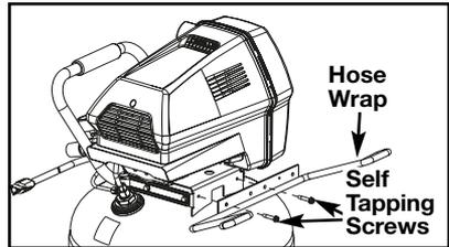
**CAUTION** DO NOT use hose wrap as a handle to push, pull, or lift air compressor.
