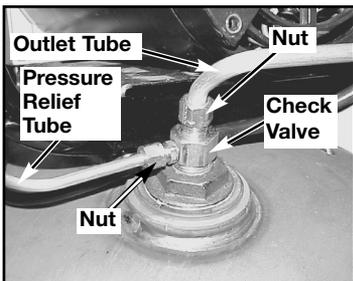
5. Using an adjustable wrench, loosen pressure relief tube nut at air tank and pressure switch. Carefully move pressure relief tube away from check valve.
