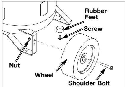
**CAUTION** It will be necessary to brace or support one side of the air compressor when installing the wheels because the compressor will have a tendency to tip.
