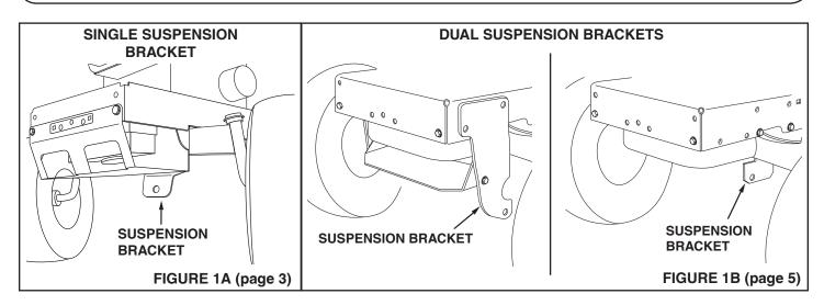
Look under the front of your tractor (Figure 1A & 1B). If there is a single mower deck suspension bracket located underneath the middle of the front axle, continue on to INSTRUCTIONS FOR SINGLE SUSPENSION BRACKET TRACTORS on page 3. If your tractor does not have a mower deck suspension bracket underneath the middle of the front axle, skip to INSTRUCTIONS FOR DUAL SUSPENSION BRACKET TRACTORS on page 5.
