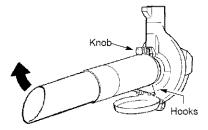
When converting back to the blower feature, make sure latch on the vacuum inlet cover is securely fastened.
