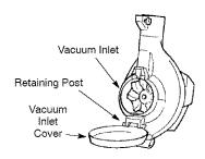
Place the hooks on the vacuum tube on the retaining posts; pivot tube into position. Secure vacuum tube by turning the knob clockwise until tight.
