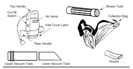
The **ON/OFF SWITCH** is used to activate the motor.
