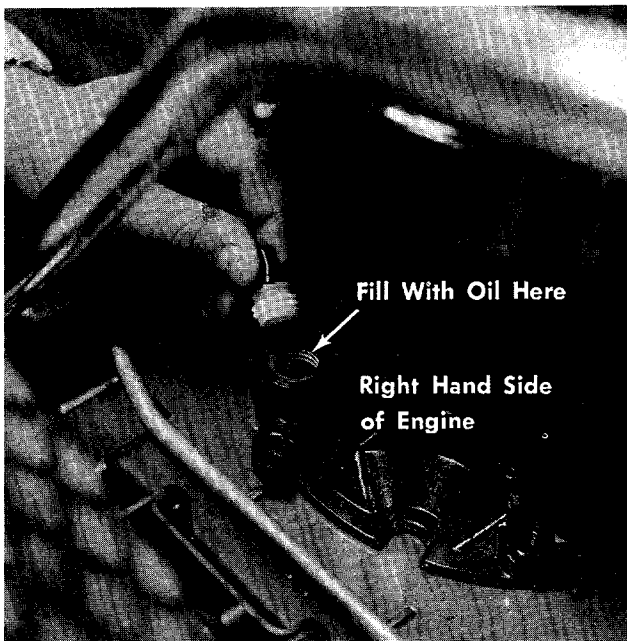
FIGURE 27. OIL FILL LOCATION
