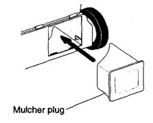
**ACAUTION:** Do not run your lawn mower without mulcher plug in place or approved clipping deflector or grass catcher in place. Never attempt to operate the lawn mower with the rear door removed or propped open.
