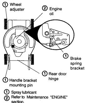
**IMPORTANT:** Do not oil or grease plastic wheel bearings. Viscous lubricants will attract dust and dirt that will shorten the life of the self lubricating bearings. If you feel they must be lubricated, use only a dry, powdered graphite type lubricant sparingly.
