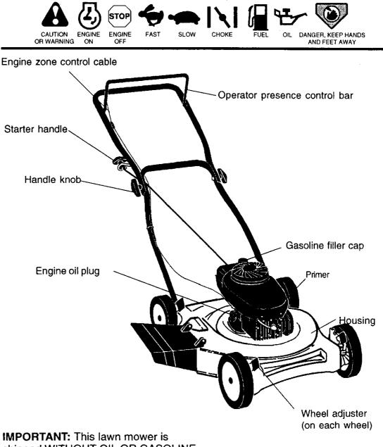
shipped WITHOUT OIL OR GASOLINE in the engine.
