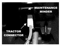
Disconnect tractor electrical connector from Maintenance Minder.
