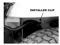
**IMPORTANT:** Do not kink hoses exiting the power unit. Leave enough excess for a generous bend in the supply lines when assembling clip to tractor.
