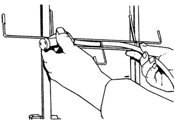
Cut tie wrap from high pressure hose. Connect high pressure hose to gun with either two adjustable wrenchs or one 11/16" and one 7/8" wrench.
