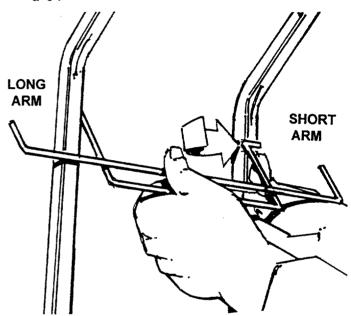
Cut tie wrap on chemical injection tube. Remove chemical injection filter, thread chemical tube through the wire form and reinsert filter into tube.
