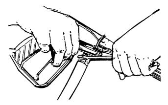
Remove plastic cap and connect high pressure hose to pump.
