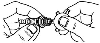
Install spark plug, tighten securely.
