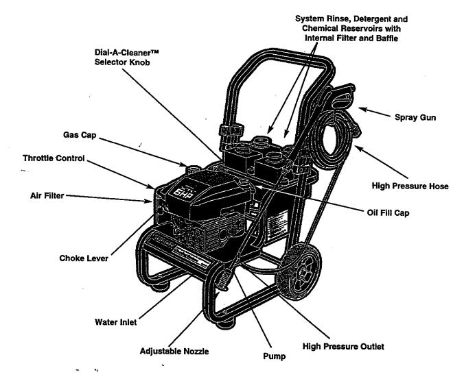
Adjustable Nozzle - Adjust for high or low pressure; narrow or fan spray.
