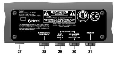
**27: FUSE:** The fuse protects the amplifier from damages caused by a faulty AC power source and/or other problems. If the fuse opens, replace it ONLY with the same size and type. If fuses continue to fail, check the AC source – if the source is okay, contact your Crate dealer for service information.
