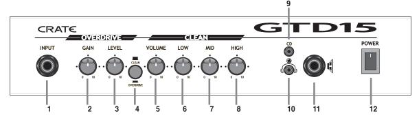
**1. INPUT:** Use this jack to connect your guitar to the amplifier by means of a shielded instrument cable.
