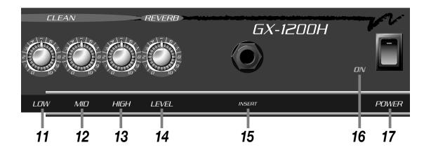
**15: INSERT:** Connect an external effects device via this jack. Use a stereo 1/4" male Y-cord: ring = send, tip = return, sleeve = ground. See the illustration on the panel to the right for more information
