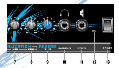
**9: REVERB LEVEL:** Use this control to adjust the amount of reverberationl: in its full counter clockwise position the signal will be "dry" (without any reverb). As you rotate the control clockwise the amount of reverberation increases.
