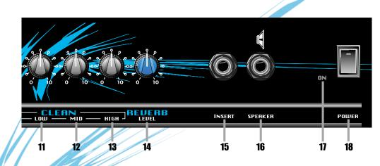
17: ON LED: This LED will illuminate when power is applied to the amplifier.
