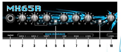
1: INPUT: Use this 1/4" jack to connect your guitar to the amplifier by means of a shielded instrument cable.
