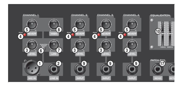
**1. MIC IN:** Use this balanced XLR jack to connect a low impedance balanced microphone signal to Channel 1 of the amplifier by means of a shielded microphone cable.
