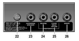
**22: FUSE:** The fuse protects the amplifier from damages caused by a faulty AC power source and/or other problems. If the fuse opens, replace it ONLY with the same size and type. If fuses continue to fail, check the AC source – if the source is okay, contact your Crate dealer for service information.
