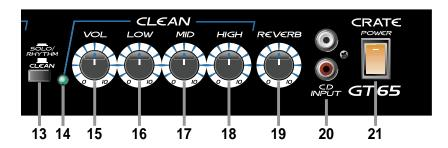
**21: POWER:** Use this switch to turn the amplifier on (top of the switch depressed) and off (bottom of the switch depressed). The switch illuminates when the power is on.
