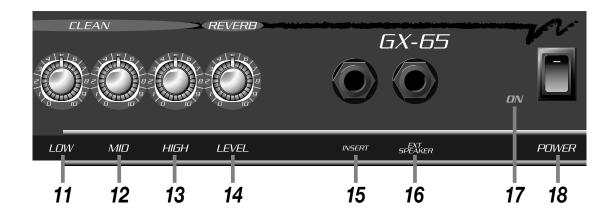
**15: INSERT:** Use this jack to connect an external effects device to the amplifier. Use a stereo 1/4" male Y-cord: ring = send, tip = return, sleeve = ground. See the illustration to the right for more information.
