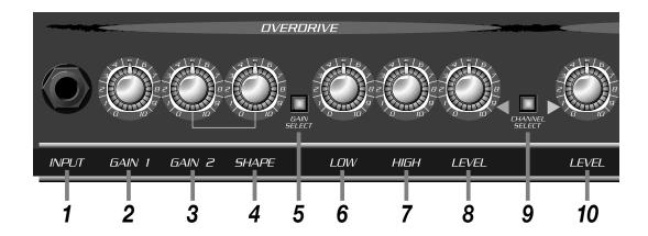
**1: INPUT:** Connect your guitar here by means of a shielded instrument cable.
