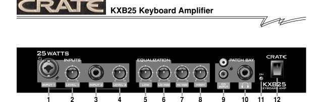
**1. INPUT 1:** Use this jack to connect a high or low impedance microphone to the amplifier by means of a shielded instrument cable. The signal level at this jack is controlled by the Level 1 knob (#2).
