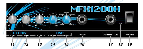
the high frequency output. Rotating the control clockwise increases the high frequency output. The High control provides a range of 28dB of boost or cut at 10kHz.
