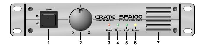
**1: POWER SWITCH:** This switch applies AC power to the amplifier. The amp is on when the top of the switch is depressed, off when the bottom of the switch is depressed. The Power LED indicator (#3) illuminates when the amplifier is on.
