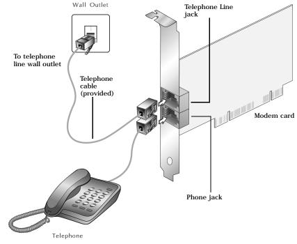
Figure 2-3 Connecting the telephone line to your modem.
