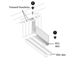
Figure 2-2 Aligning the card against the slot.
