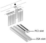
Figure 2-1 Removing a metal plate
