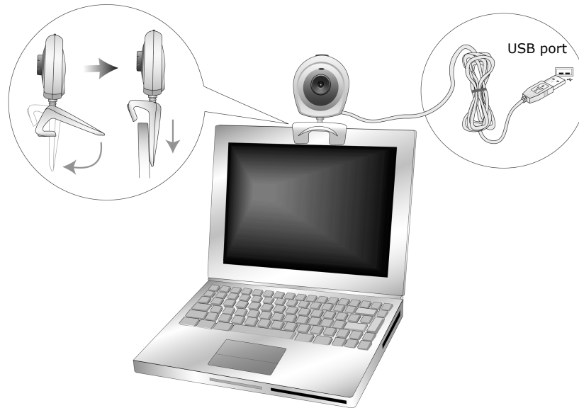
Figure 1-3: Connecting Creative WebCam Pro eX to your laptop.
