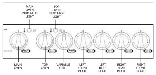
**Control Knobs** The knobs for the hotplates can be rotated in either direction to provide variable heat control, the Main Oven and Top Oven knobs can only be rotated clockwise from the **Off** position.
