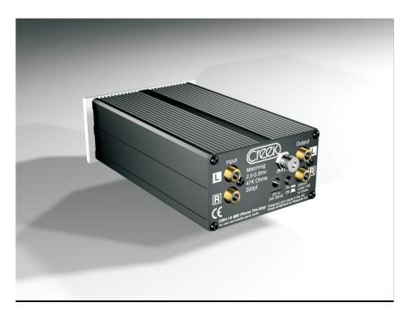
Connect the OBH 18 to the input of your amplifier with a stereo RCA inter-connect cable. If using a Creek integrated amplifier connect to the first input.
