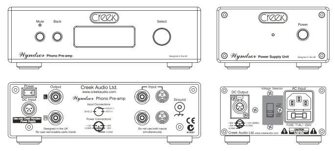
A DIN plug is provided to enable the correct cable to be produced for balanced input connection. The wiring configuration is noted on the rear panel. Please consult your dealer if in any doubt. Additional information can be accessed from the FAQ section of the Creek Audio website.
