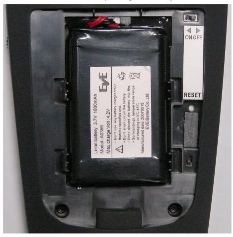
TPMC-4XG-BTP in Battery Compartment of TPMC-4XG-B
