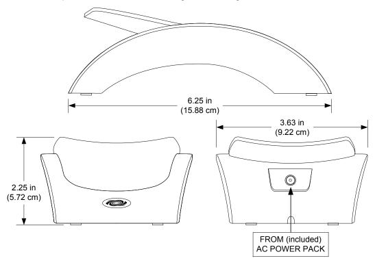
**WARNING:** To avoid possible physical harm, damage to the TPMC-4XG-DS-B or touchpanel, use only the included power pack (100-240 VAC, 50/60 Hz) when charging.
