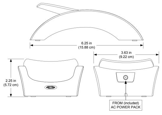
**WARNING:** To avoid possible physical harm, damage to the TPMC-4XG-DS or touchpanel, use only the included power pack (100-240 VAC, 50/60 Hz) when charging.
