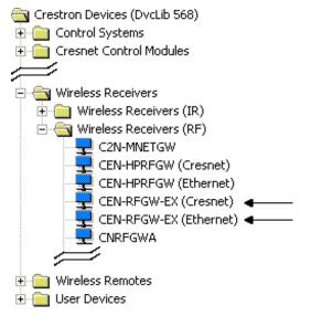
• The system tree of the control system displays the device in the appropriate slot with a default Net ID or IP ID, as shown in the following illustration.
