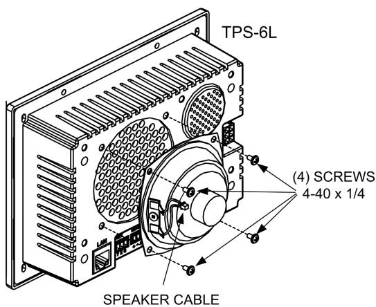
2. Refer to the following illustration and plug the two-conductor speaker cable into the mating connector on the speaker box assembly. Then plug the six-wire cable from the speaker box assembly into the mating connector on the rear of the touchpanel.
