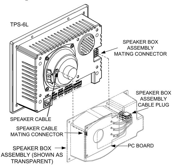
3. Use a #2 Phillips screwdriver to secure the speaker box to the touchpanel with six supplied screws. Refer to the following illustration.
