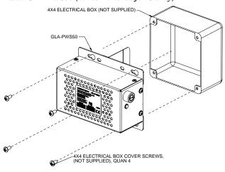
**NOTE:** The GLA-PWS50 should never be installed with the label facing down.
