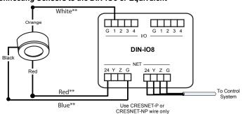
\*The following Crestron devices may be used to integrate the sensors into a Cresnet system by following the schematic shown
