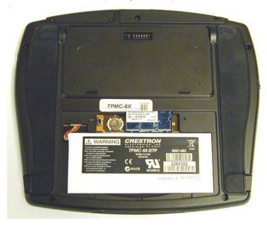
TPMC-8X-BTP in Battery Compartment of TPMC-8X
