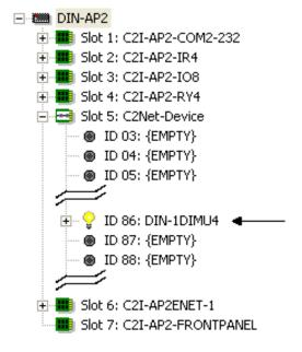
• Additional DIN-1DIMU4 devices are assigned different Net ID numbers as they are added.
